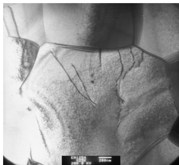
Figure 17 TEM micrograph of gadolinia doped ceria showing dislocations within a grain.
