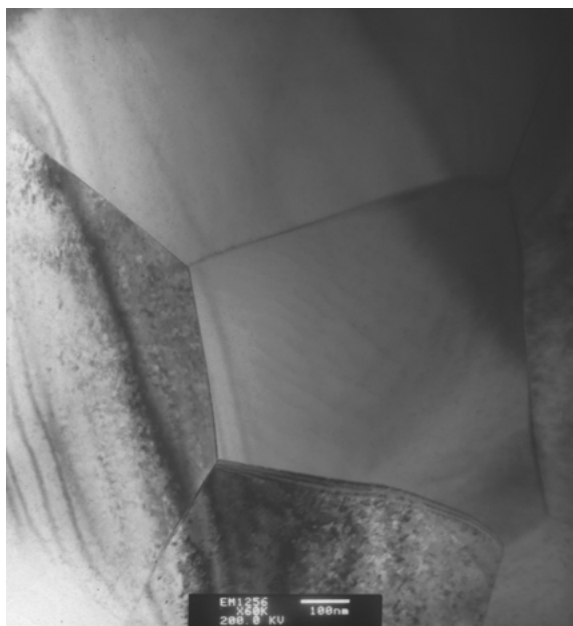
Figure 15 TEM micrograph of gadolinia doped ceria showing grain sizes and grain boundaries.
